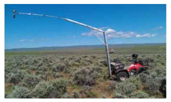
An ATV is mounted with a DSLR camera on an extended boom to shoot high-resolution images of ground cover. Photo courtesy of Open Range Consulting, Inc.
